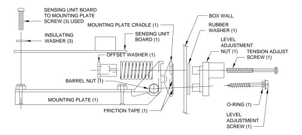
**IMPORTANT:** With early control boxes, the mounting plate hole in the control box may not be large enough. Use a step drill bit to enlarge the hole to 7/8". DO NOT use a standard drill bit. This will most likely damage the control box. When drilling is complete, make sure all metal chips are removed from the box and that no metal chips are on the control box P.C. board. Metal chips on the P.C. board may cause damage to the board.
