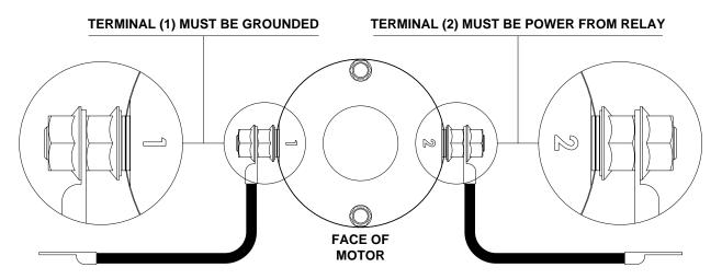
TERMINALS ARE NUMBERED ON THE FACE OF THE MOTOR TIGHTEN TERMINAL NUTS TO 44 IN·LBS, MAX
