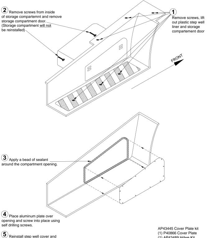
Reinstall step well cover and storage compartment door.
