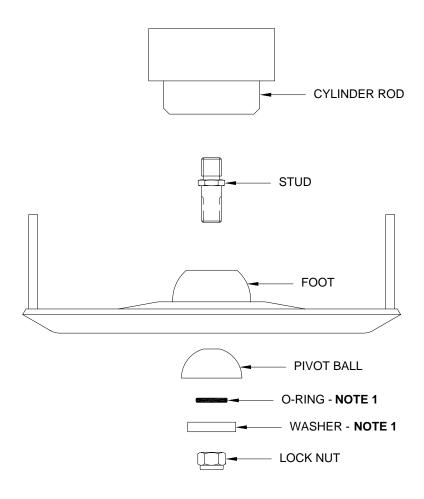
**NOTE 1:** O-RING AND WASHER ARE ONLY USED WITH POWER-EXTEND / POWER-RETRACT (DOUBLE-ACTING) JACKS.
