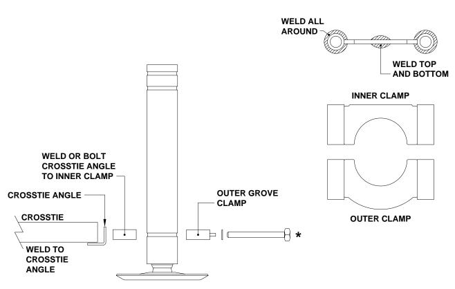
\* LONG BOLTS AND NUTS ARE USED WITH BOLT THRU CLAMP SHORT BOLTS ARE USED WITH WELD ON CLAMP
