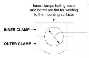
The smaller diameter of a groove clamp will fit in a barrel groove, but will not fit around the full diameter of the barrel. The upper groove clamp keeps the jack at the proper mounting height and caries the entire vertical load for the jack. There are two upper grooves on the cylinder allowing the jack to be raised or lowered to achieve optimal mounting height. The lower groove prevents the crosstie from slipping up or down.
