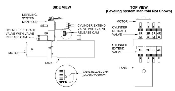
IMPORTANT: Open both the Cylinder Extend and Cylinder Retract valves for a room to release pressure before replacing one or both valves for that room. Turn the Valve Release Nuts NO MORE THAN 4 1/2 full turns counter clock wise to open the valves. Remember to close the valve(s) after the repair is complete. Tighten the Valve Release Nuts snug only. DO NOT over tighten.
