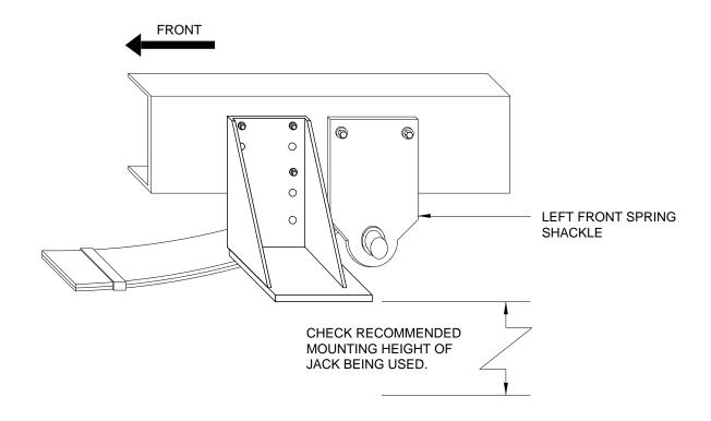
**NOTE:** USE 4 BOLTS TO MOUNT BRACKET. THE MINIMUM SPACING VERTICALLY BETWEEN BOLTS IS 3 INCHES.
