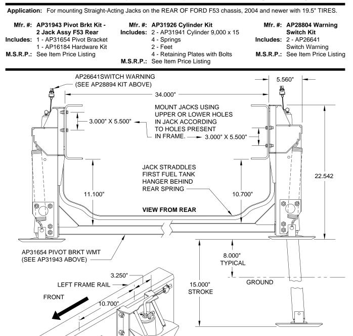
NOTE: 2004 MOTOR HOMES MAY HAVE 2003 OR 2004 CHASSIS. THE 10TH POSITION OF THE VIN CODE WILL BE A "3" OR A "4" TO DESIGNATE 2003 OR 2004 CHASSIS.
