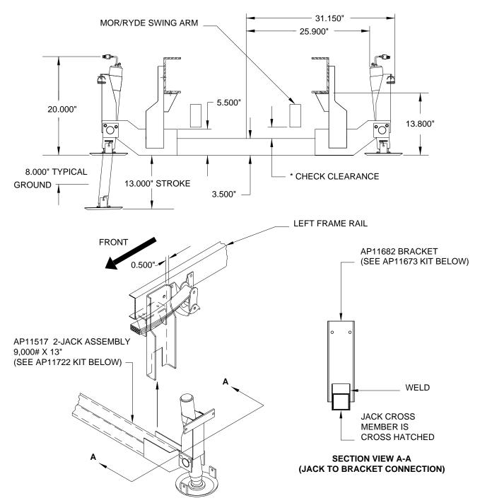
THE ABOVE DRAWING SHOWS JACKS MOUNTED OUTBOARD ON THE REAR SPRING HANGERS ON A FORD F53.
