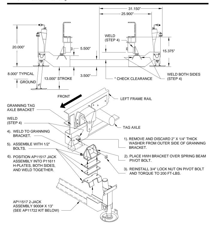
ABOVE DRAWING SHOWS JACKS MOUNTED OUTBOARD OF THE REAR SPRING HANGERS ON A CHEVROLET P30.
