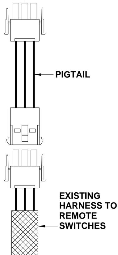
Unplug existing harness and insert pigtail between Touch Panel end existing harness.
