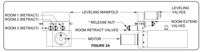
\* DO NOT loosen the Release Nut (Counter Clockwise) more than 4 and 1/2 turns. DO NOT over tighten when closing.
