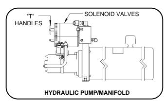
3. Open the SOLENOID VALVES by turning the "T" HANDLES counterclockwise.
