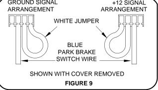
+12 PARK BRAKE: Eliminate the diode arrangemnent at the end of the blue park brake wire. (FIGURE 8) Splice the blue wire directly onto the wire from the park brake switch. Soldering with shrink tube is the preferred way to make this connection. A different park brake harness may be ordered for +12 park brake installations or the original plug can be rewired to work corrrectly. (See FIGURE 9)
