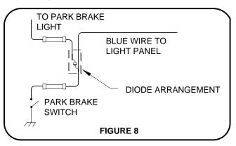
+12 PARK BRAKE: Eliminate the diode arrangemnent at the end of the blue park brake wire. (FIGURE 8) Splice the blue wire directly onto the wire from the park brake switch. Soldering with shrink tube is the preferred way to make this connection. Remember, a different control box is needed if the signal is +12.
