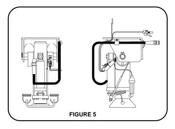
**9000# KICK DOWN JACK-** When connecting the hose to the jack, the hose should go in the upper left-hand corner, over the pivot area and down the front of the jack. After connecting the hose to the fitting, the hose should be clamped with a 1/4" bolt to the left side of the pivot bracket. Be sure the hose is snug against the jack in the retracted (horizontal) position.
