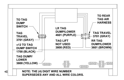
During the normal travel mode, the Tag Travel valves are tied electrically to the Front and Rear air manifold Travel valves. The Travel Fuse also protects the Tag Manifold Travel valves.
