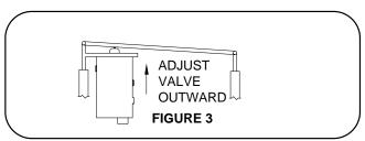
If the valve side of the room is moving at a greater distance from the vehicle (FIGURE 3) turn the adjusting bolt clockwise 1 turn. **NOTE** : If the difference is minor, less than 1 turn may be appropriate. Extend the room an additional 12 inches. Retract the room that 12 inches and check the measurement. Repeat this procedure as necessary. The difference in the measurement should be 1/2 an inch or less. Tighten the mounting bolts and adjusting lock nut when the adjustment is complete.
