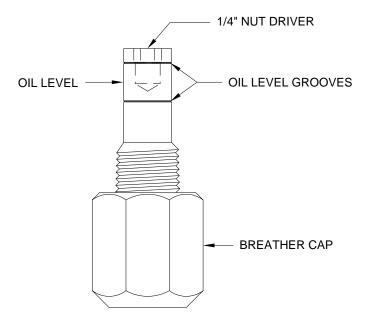
IMPORTANT: PRIOR TO REMOVING THE BREATHER CAP, EITHER TO CHECK THE OIL LEVEL OR TO USE THE 1/4" NUT DRIVER, CLEAN ANY DEBRIS FROM THE TOP OF THE RESERVOIR. BEFORE RETURNING THE BREATHER CAP TO THE RESERVOIR, REMOVE ANY PAINT CHIPS OR OTHER DEBRIS FROM THE DIPSTICK INCLUDING DEBRIS INSIDE THE 1/4" NUT DRIVER.
