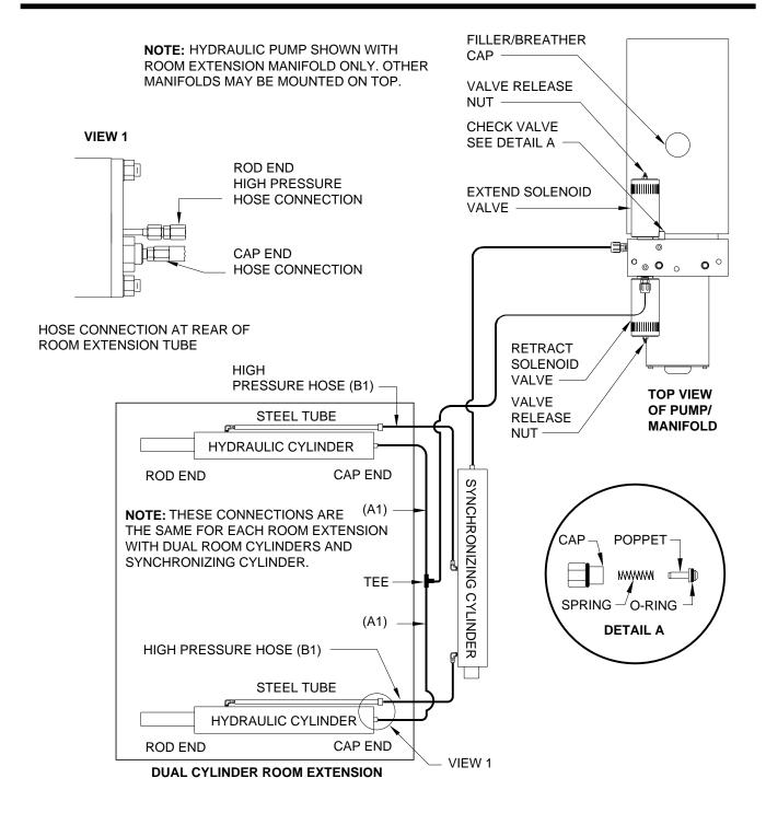
**IMPORTANT:** THE LINES (A1) BETWEEN THE CAP END OF THE HYDRAULIC CYLINDERS AND THE TEE MUST BE THE SAME LENGTH AND DIAMETER. THE LINES (B1) BETWEEN THE ROD END OF THE HYDRAULIC CYLINDERS AND THE SYNCHRONIZING
