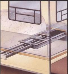
HWH's unique SpaceMaker single cylinder room extension increases the size of a room by up to 34 inches.
