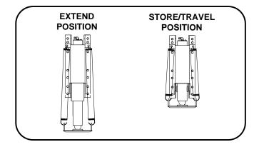
**CAUTION:** DO NOT MOVE THE VEHICLE WHILE THE LEVELING JACKS ARE STILL IN CONTACT WITH THE GROUND OR IN THE EXTEND POSITION. THIS VEHICLE IS EQUIPPED WITH STRAIGHT-ACTING JACKS. MOVING THE VEHICLE WITH THE LEVELING JACKS EXTENDED CAN CAUSE SEVER DAMAGE TO THE JACKS AND OR THE VEHICLE AND CREATE A DRIVING HAZARD. DO NOT RELY SOLELY UPON WARNING LIGHTS. IT IS THE OPERATOR'S RESPONSIBILITY TO CHECK THAT ALL JACKS ARE FULLY RETRACTED INTO THE STORE/TRAVEL POSITION.
