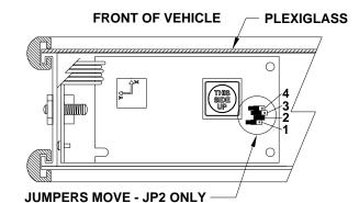
NOTE: AFTER MOVING THE JUMPERS, REMOVE AND REAPPLY +12 POWER FOR THE CONTROL BOX. THIS WILL "RE-BOOT" THE SENSING UNIT.
