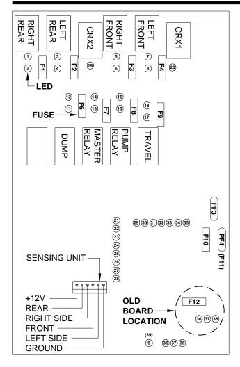
NOTE: FOR DETAILED INPUT / OUTPUT INFORMATION ABOUT PIN CONNECTIONS SEE ELECTRICAL CONNECTION DIAGRAM - CONTROL BOX CONNECTION INFORMATION.
