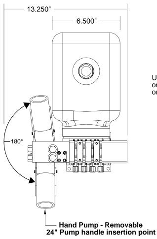
Up to four hydraulic switch controls will operate up to four one way jacks, four two way jacks or four room extensions or a combination there of.
