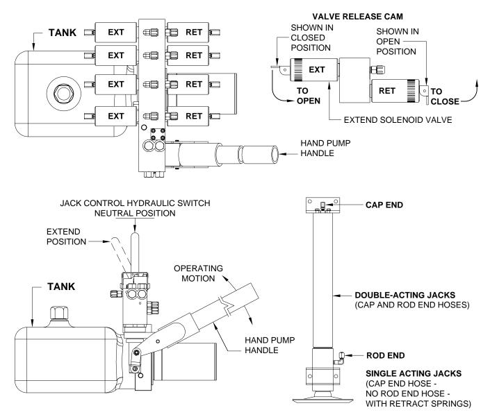
To prime the hand pump, it will be necessary to remove a hose from one of the jacks. One of the front jacks would be best, but use the easiest hose to get to.
