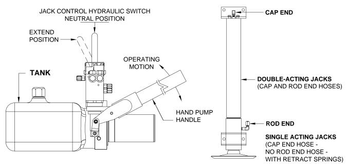
To prime the hand pump, it will be necessary to remove a hose from one of the jacks. One of the front jacks would be best, but use the easiest hose to get to.
