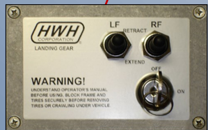
Weather resistant metal box with sealed toggle switches for long life
