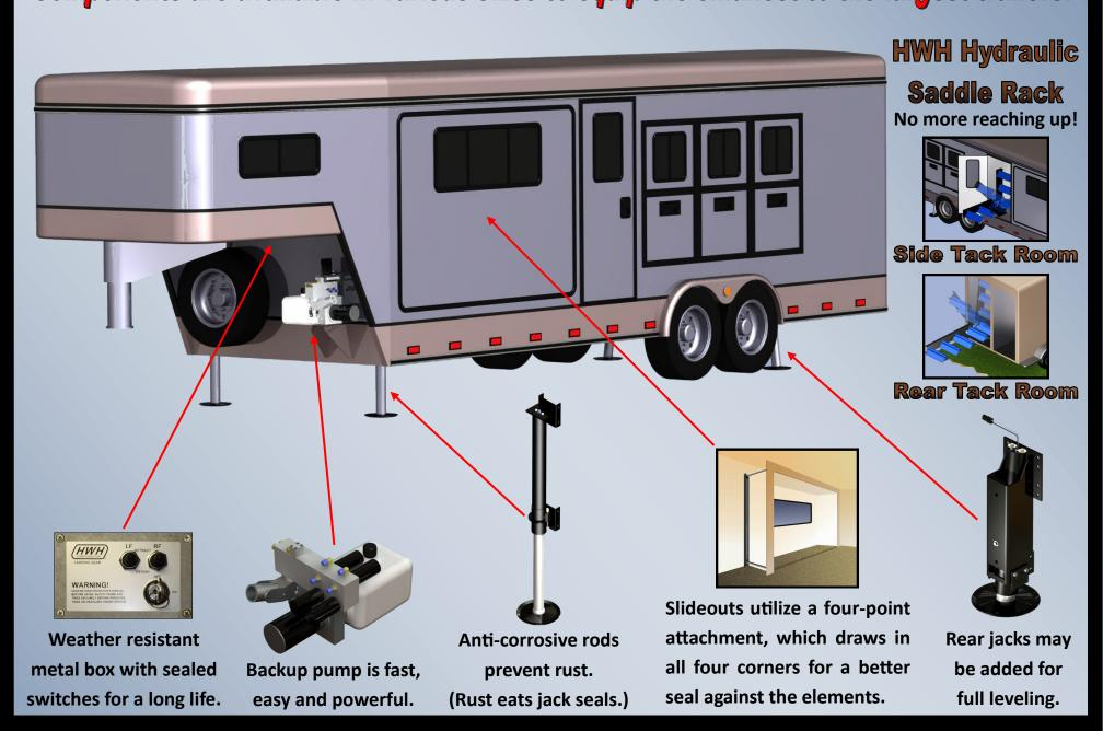
Only one multi-purpose power unit is needed to run all HWH equipment. Landing Gear | Leveling System | Room Extension Systems | Saddle Rack
