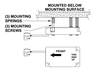
BOTTOM VIEW OF LEVEL SENSING UNIT
