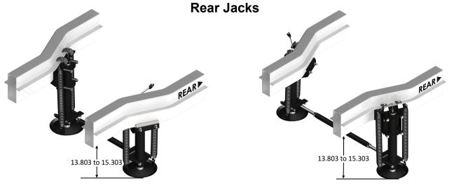
Rear Jacks Mounted Inboard------OR------Rear Jacks Mounted Outboard
