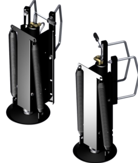
AP37524 Jack Kit Two Straight-Acting (Power-Extend/Spring-Retract) Jacks with a lifting capacity of 6,000 lbs. per jack on the rear (Fits five cylinder diesel)
