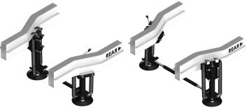
AP52759 Rear Jack OR AP52759 Rear Jack Mounted Inboard Mounted Outboard
