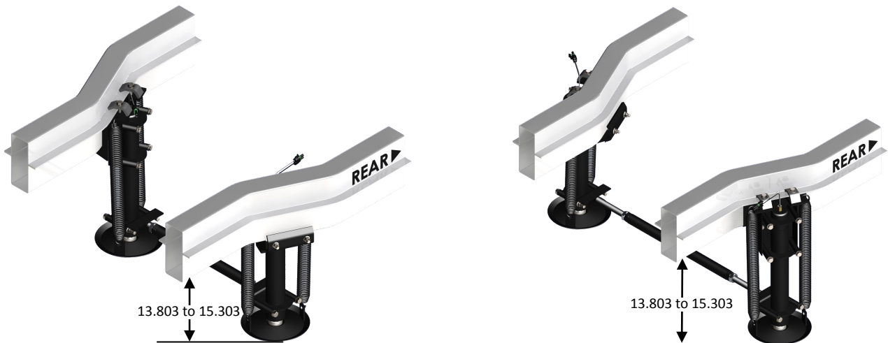
Rear Jacks Mounted Inboard-----OR-----Rear Jacks Mounted Outboard
