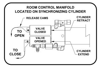
If the pump manifold is equipped with an auxiliary hand pump, you may be able to retract the room by opening only the room retract valve (as labeled by the wiring harness) and operating the hand pump, refer to the AUXILIARY HAND PUMP OPERATION page for instructions on the use of the hand pump and valves equipped with a release cam. If the room cannot be retracted with the hand pump, it will be necessary to use the lift bolts and room retract screws.
