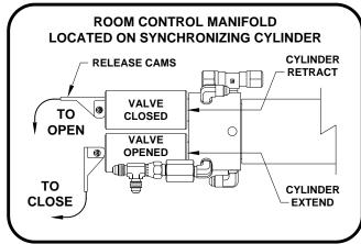
If the pump manifold is equipped with an auxiliary hand pump, you may be able to retract the room by opening only the room retract valve (as labeled by the wiring harness) and operating the hand pump, refer to the AUXILIARY HAND PUMP OPERATION page for instructions on the use of the hand pump and valves equipped with a release cam. If the room cannot be retracted with the hand pump, it will be necessary to use the lift bolts and room retract screws.
