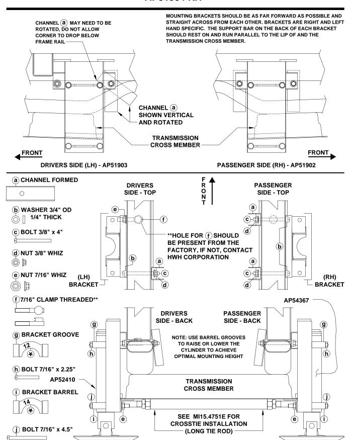
\* BRACKETS ARE DIAMETER SPECIFIC. THE SMALLER DIAMETER MUST BE USED IN A GROOVE. THE LARGER DIAMETER MUST BE USED AROUND THE BARREL.
