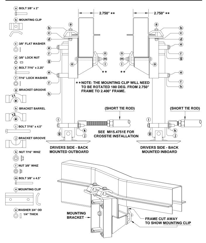
BRACKETS MUST BE MOUNTED BOTH OUTBOARD OR BOTH INBOARD OF THE FRAME.
