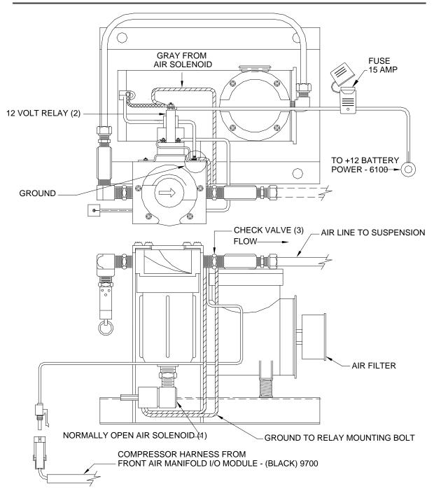
The control box sends a +12 signal to the normally open 12 volt relay. The 12 volt relay (2) will energize and the compressor will run. The normally open air solenoid (1) will close allowing the compressor to build pressure.
