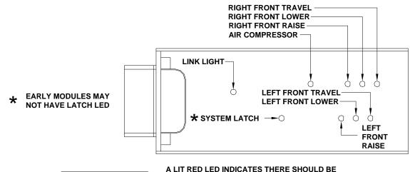
A LIT RED LED INDICATES THERE SHOULD BE +12 VOLTS ON THE CORRESPONDING WIRE.
