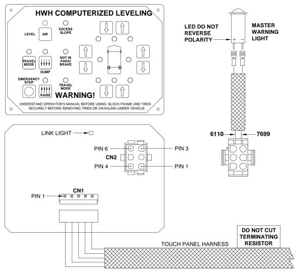
NOTE: THERE IS A 120 OHM TERMINATING RESISTOR AT EACH END OF THE TOUCH PANEL HARNESS. DO NOT REMOVE, CUT OR MODIFY THE HARNESS.
