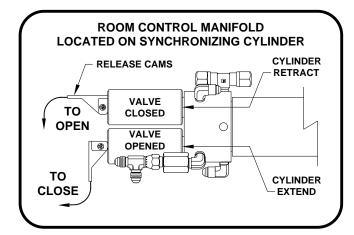
NOTE: The valve release cam might be rotated in any direction on the valve. Pushing the release cam in the wrong direction could damage the valve.
