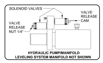
3. Open Nut Style Solenoid Valves by slowly turning the valve release nut counter clockwise using a 1/4" nut driver.
