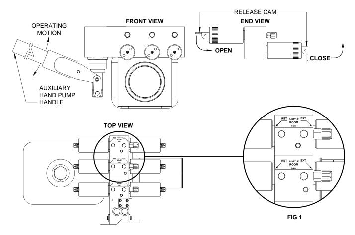
NOTE: Each hydraulic function requires a pair of solenoid valves one each for the extend and retract procedures. The number of functions and the items controlled by each pair of solenoid valves will very for each system. The diagrams shown on this page represent a (3) function system of (3) rooms as indicated by the labels shown in FIG 1. Use the labels specific to your system when following these procedures.
