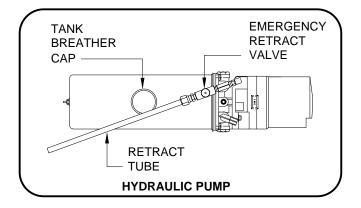
2. Remove the tank breather cap and place the retract tube in the breather cap opening.
