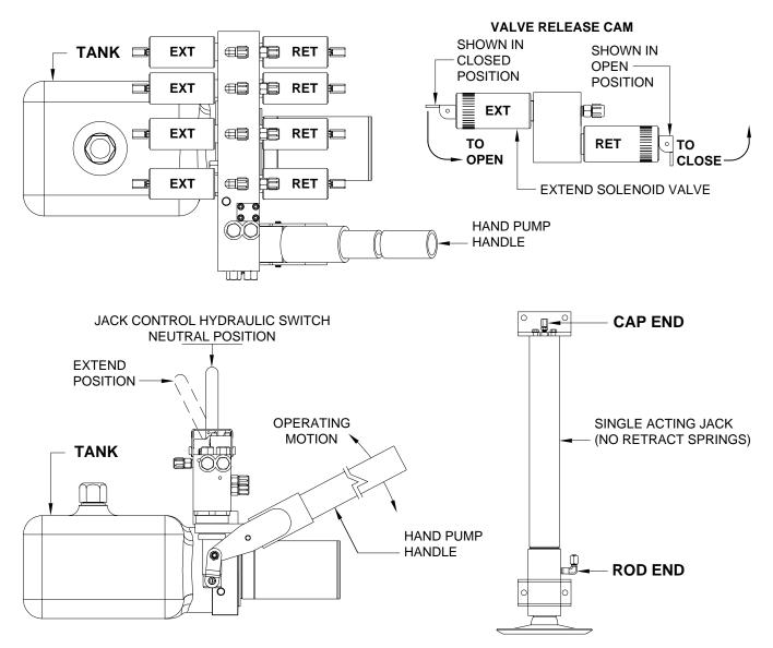
To prime the hand pump, it will be necessary to remove a hose from one of the jacks. One of the front jacks would be best, but use the easiest hose to get to.
