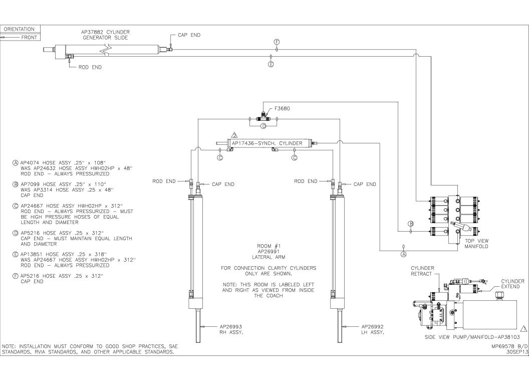
NOTE: HOSES (C) AND (D) ARE INCLUDED WITH THE ROOM EXTENSION MECHANISM
