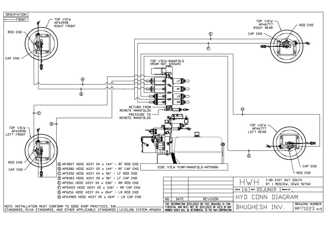
NOTE: HOSES (E) AND (F) ARE INCLUDED WITH THE ROOM EXTENSION MECHANISM
