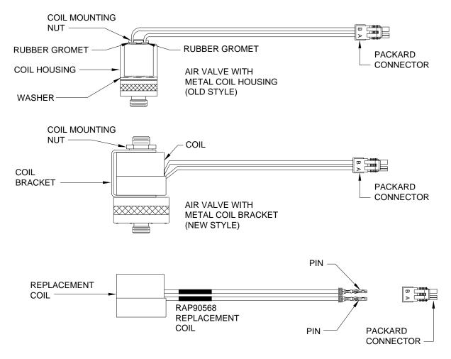
The RAP90568 replacement coil is supplied with the 2-pin Packard connector loose. The pins must be insterted into the Packard connector AFTER the coil has been installed. Either wire can be inserted into the A or B side of the connector. Pull gently on the wires after inserting the pins to insure the pins are properly seated in the Packard connector.
