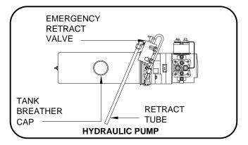
2. Remove the tank breather cap and replace the retract tube in the breather cap opening.
