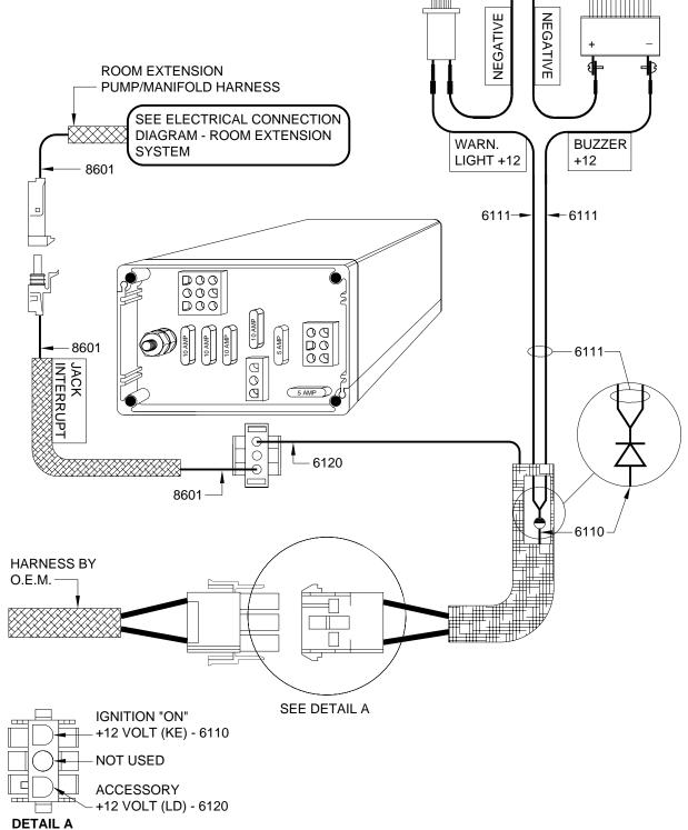
**ELECTRICAL CONNECTION DIAGRAM 310 SERIES LEVELING SYSTEM WITH ROOM EXTENSIONS** POWER HARNESS AND MASTER WARNING INDICATORS
