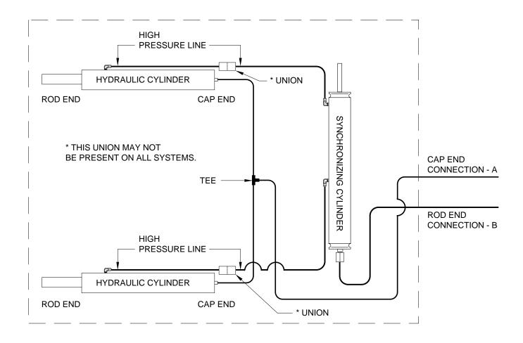
**IMPORTANT:** THE TWO 3/16" HIGH PRESSURE LINES BETWEEN THE SYNCHRONIZING CYLINDER AND THE ROD END OF THE ROOM CYLINDERS MUST BE EQUAL IN LENGTH AND DIAMETER. THE HYDRAULIC LINES BETWEEN THE CAP END OF THE ROOM CYLINDERS AND WHERE THEY TEE TOGETHER MUST BE OF EQUAL LENGTH AND DIAMETER.
