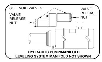
3. Open the Solenoid Valves by slowly turning the valve release nuts counter clockwise using the 1/4" nut driver supplied.
