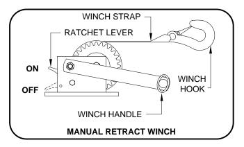
5. Slowly winch the room in by turning the WINCH HANDLE clockwise. The RATCHET LEVER should produce a loud, sharp, clicking noise.
