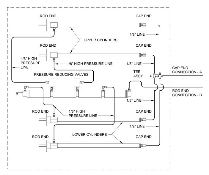
**IMPORTANT:** THE TWO LINES BETWEEN THE CAP END OF THE LOWER CYLINDERS AND THE TEE ASSEMBLY MUST BE THE SAME LENGTH AND DIAMETER.
