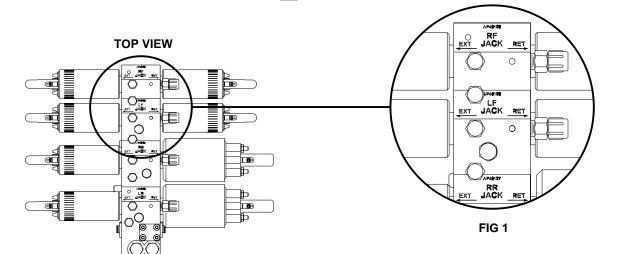
NOTE: Each hydraulic function requires a pair of solenoid valves one each for the extend and retract procedures. The number of functions and the items controlled by each pair of solenoid valves will vary for each system. The diagrams shown on this page represent a (4) function system indicated by the labels shown in FIG 1. Use the labels specific to your system when following these procedures.
