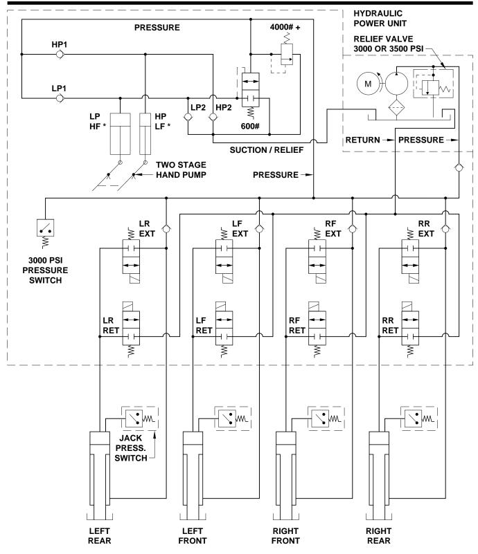
\* LPHF - LOW PRESSURE HIGH FLOW \* HPLF - HIGH PRESSURE LOW FLOW NOTE: DO NOT USE SCHEMATIC FOR CONNECTION INFORMATION. REFER TO SPECIFIC CONNECTION DIAGRAMS FOR CONNECTION INFORMATION.
