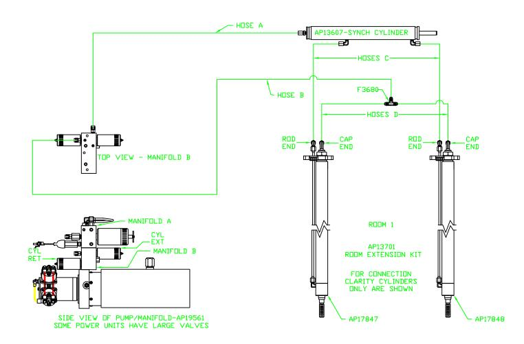
NOTE: HOSES C MUST BE HIGH PRESSURE HOSES OF EQUAL LENGTH AND DIAMETER
