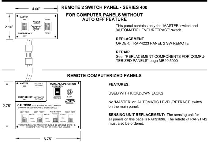
NOTE: Panels should have a tag with the part number on the back.
